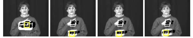
Figure 4: n -best tracking list with 450 hand hypotheses in each frame at different time stamps of a video sequence: the target object, i.e. the right and dominant-hand, is always among the active hypotheses tracking set. However, due to an abrupt movement of the dominant hand, the best path w.r.t. the tracking criterion (yellow rectangles) would track the entering non-dominant hand.
